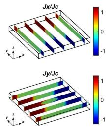
Fig. 1. Current density at a peak of a sinusoidal applied field: solution of the anisotropic bulk benchmark problem computed using a 6-film stack approximation.
