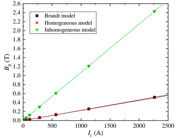
Fig. 2. Applied magnetic field strength at which a superconducting strip is no longer fully shielded,  $B_p$ , for a range of critical currents,  $I_c$ . The solid lines are linear fits to the data.
