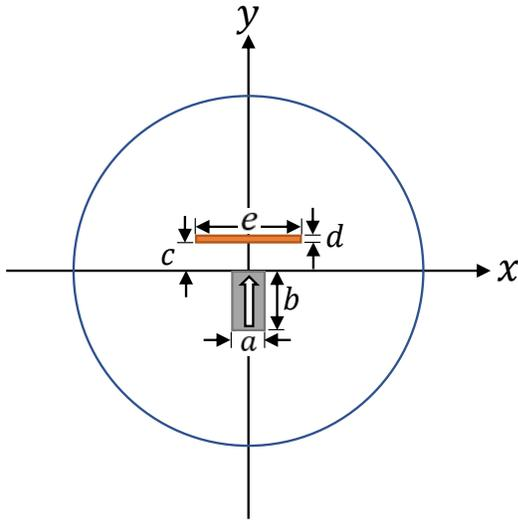
Fig. 1. Geometry of the inhomogeneous applied field model. A permanent magnet is stationary, centred under an HTS tape, and the remanent flux density of the magnet is increased.
