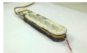
Fig. 3. Outer view of the HTS coil
