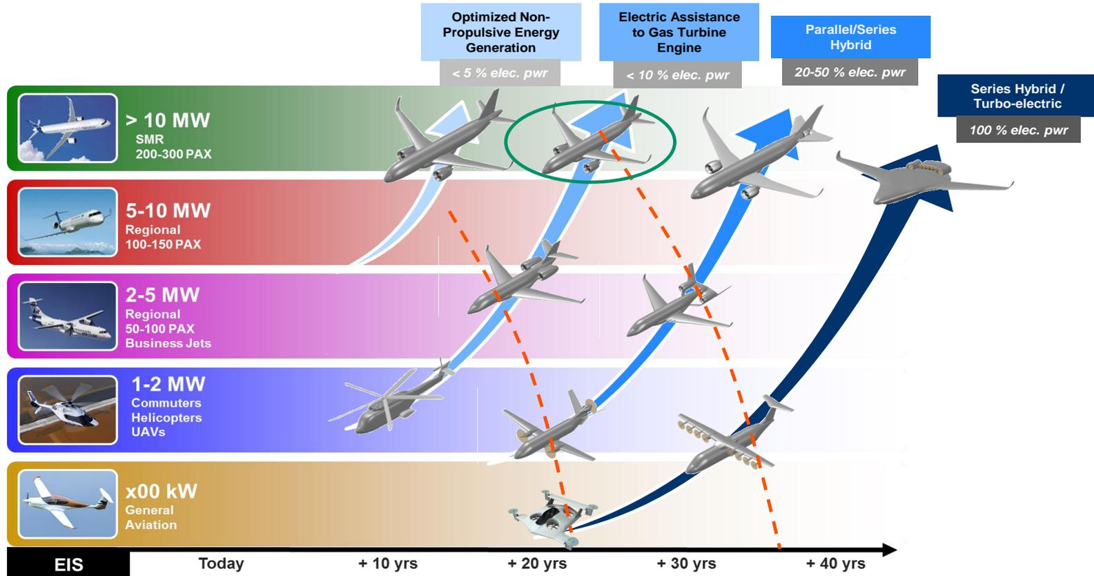
*A Step by step approach to hybridization and/or all electric propulsion*
