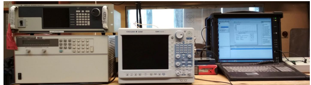
1 – PC, 2 – extension socket, 3 – Current source, 4 – current sensor, 5- scopecorder YOKOGAWA, 6 – coil, 7 – cryostat. Test bench for experimental research of HTS coils
