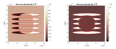
Current density distributions for the magnetization (left) and transport (right) cases. Each tape behaves differently, influence of separation, etc.
