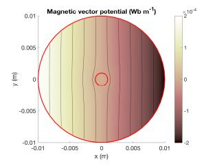
Magnetic field  $B_a$  obtained with boundary condition  $A = -B_a x$  on the outer domain
