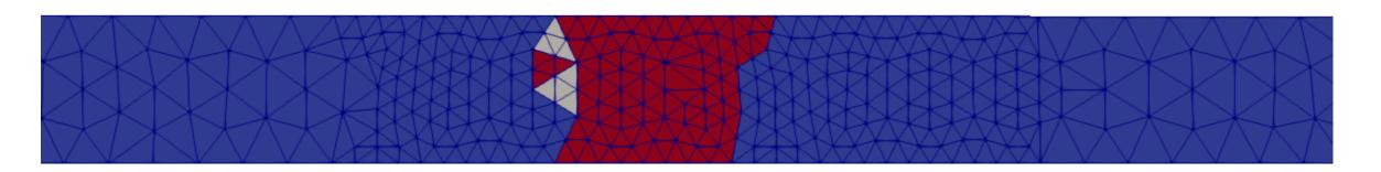
The adapted mesh and adapted interpolation order, shortly after quench initiation, is illustrated above (from top to bottom: temperature field, electric potential field and its interpolation order from 1 to 3). As can be seen the mesh is refined only around the quench location and the
