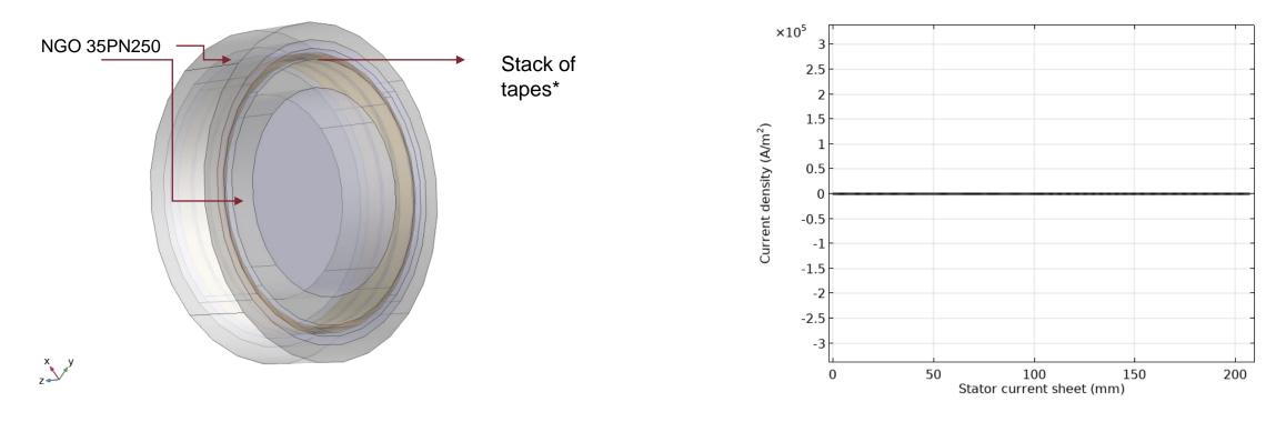
\*SuperPower advanced pinning model: 4 mm, Ic @ 0 T = 47 A Ic(B) curve from the HTS tape database @ Univ. of Wellington
